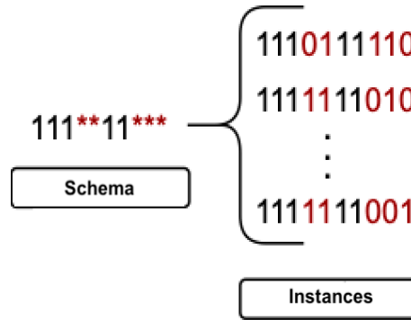
Figure 6.8: A simple example of chromosome instances which are built from a general schema.
